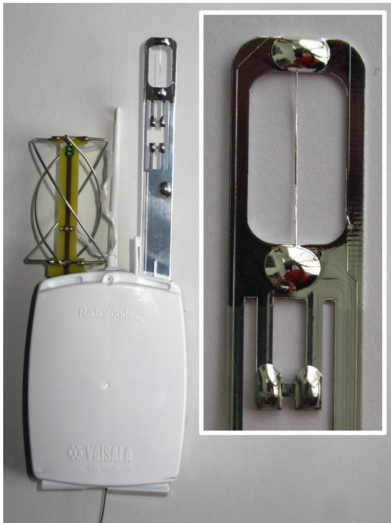
Figure 4. Photograph of the RS92 radiosonde showing the GPS antenna on the left and the sensor boom on the right. The inset shows the magnified tip of the sensor boom with the wire-shaped temperature sensor and one of the humidity sensors
